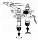
**1**. Carefully place the BA-14 over the master cylinder reservoir. Adjust the sliding plates to align the 2 rubber cones with the 2 port fittings at the bottom of the reservoir bowl.
