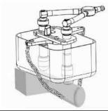
**3**. With the adjusting plates locked, wrap the security chain beneath the master cylinder. Don't run chain beneath the reservoir itself. Pull chain hand tight and secure one of the chain links in the slot. Should be snug not tight.
